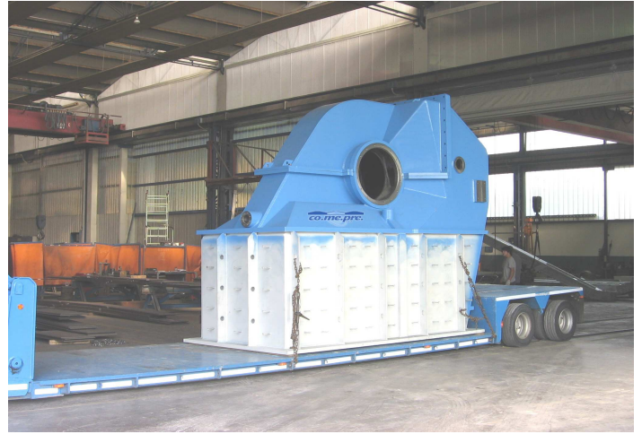
Cassa Pelton – Pelton housing – Peltongehäuse
