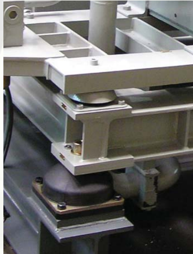
Doppelelastische Aggregate-Lagerung Double elastic mounting of engine
