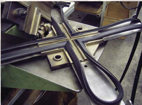
Eckenheizform zur Herstellung von Gummiprofilschnurrahmen Corner heating form for the production of co-extruded rubber profiles
