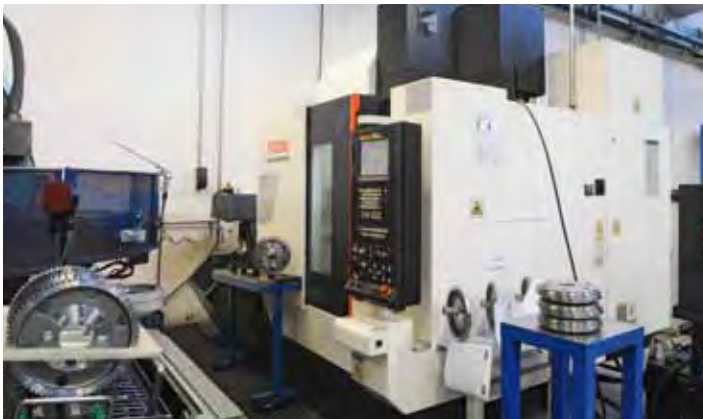
- ISOLE SUPPORTI PORTA CORONA - RING GEAR SUPPORTS MACHINING CELLS
