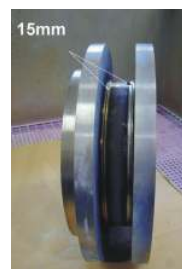
Rundnaht DN 300, 15mm tief, 15Mo3
