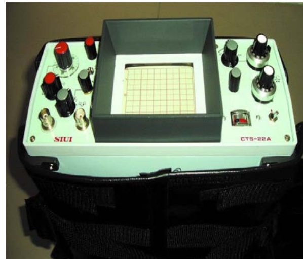
ultrasonic defect detector
