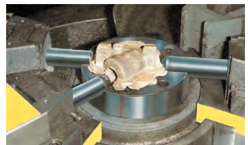
Minimizing the weight using the hollow part method
