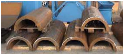
Rohrhalbschalen – Dicke 60 mm, Radius 230 mm Pipe half shelves – thickness 60 mm, radius 230 mm
