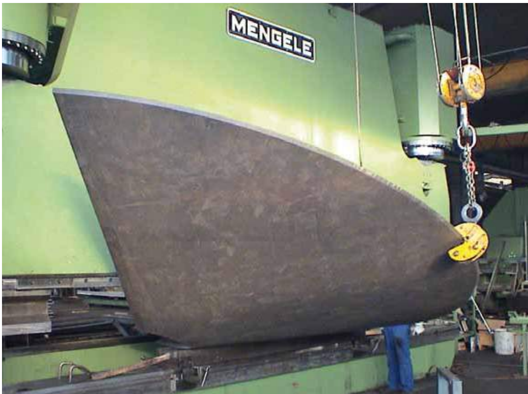
Rohrhalbschalen – Dicke 60 mm, Radius 230 mm Pipe half shelves – thickness 60 mm, radius 230 mm
