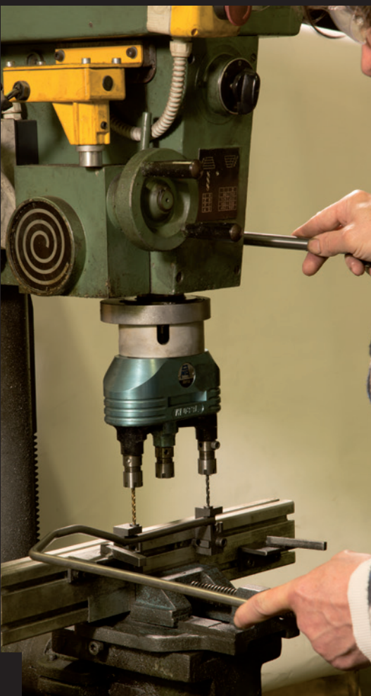
Multiple drilling operations on already bent parts
