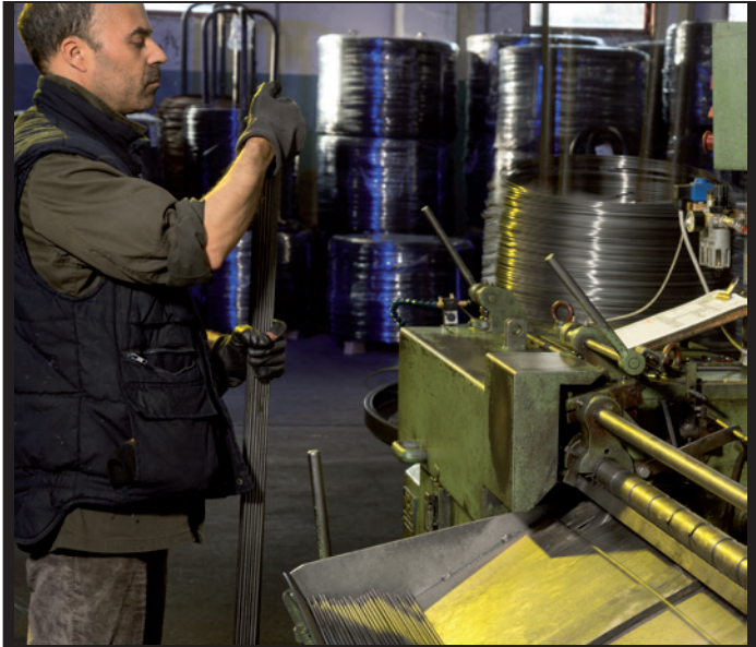
Automatic wire straightening in coils and cut to size
